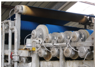
Food industry: lubrication of press ball bearings.
